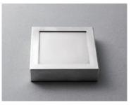
Sample: 50x50 Square Material: NAK80 Electrode material: Copper Electrode quantity: 1 Roughness: 0.12~0.15 µm
