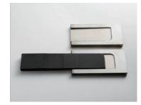
Sample: Graphite Rib Material: NAK80 Electrode material: Graphite Electrode quantity: 1 Electrode Wear: 1.98%
