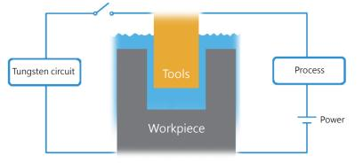
By equal discharge pulse circuit, it detects the real time Gap sparking status where it auto-adjust discharge condition to reduce electrode wear and improve discharge efficiency from rough surface to finished sparking surface.
