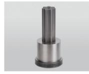
Sample: Punch Material: Tungsten Carbide Electrode material: Copper Electrode quantity: 3 Roughness: Ra 0.3 µm
