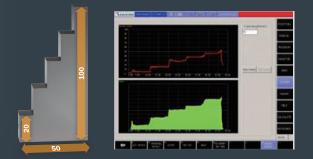
DPM is capable of detecting digital signals of sparking density, providing feedback to the CNC system and calculating the sparking size.
